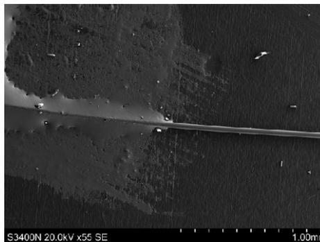
**Figure 3.7.** A 40 μm aluminum wire coated with 10 nm of gold. Good tin wettability and high-quality soldering are evident.
