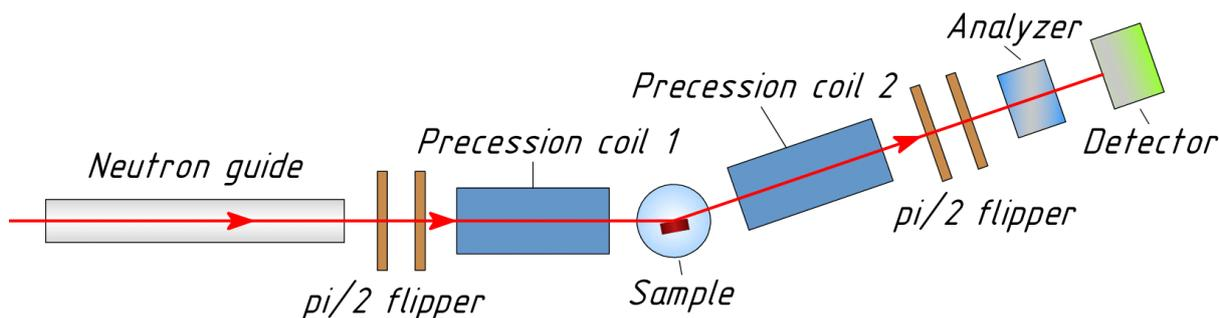
Fig. 7. NSE instrument layout
