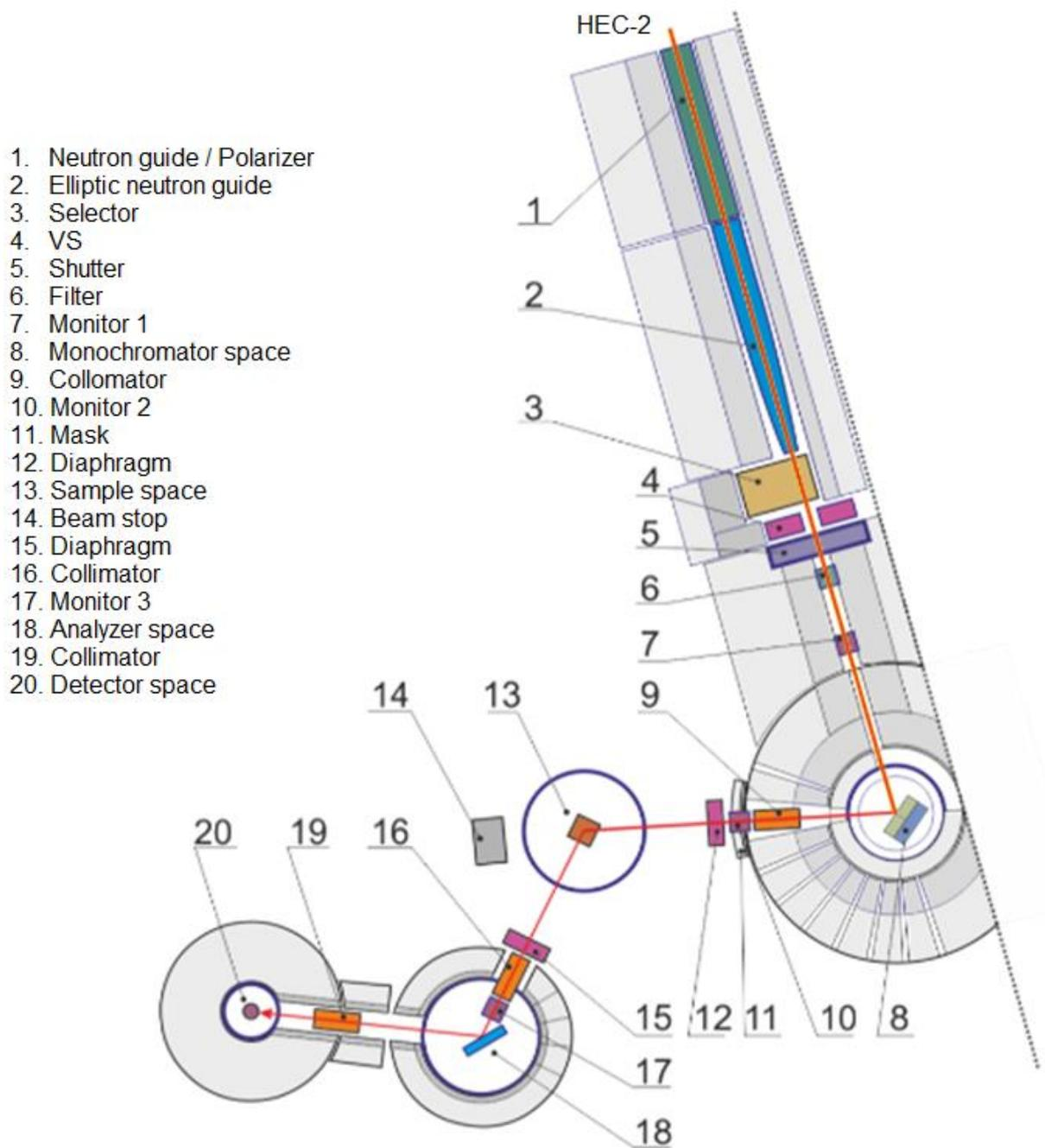
Fig. 5. TAS instrument layout
