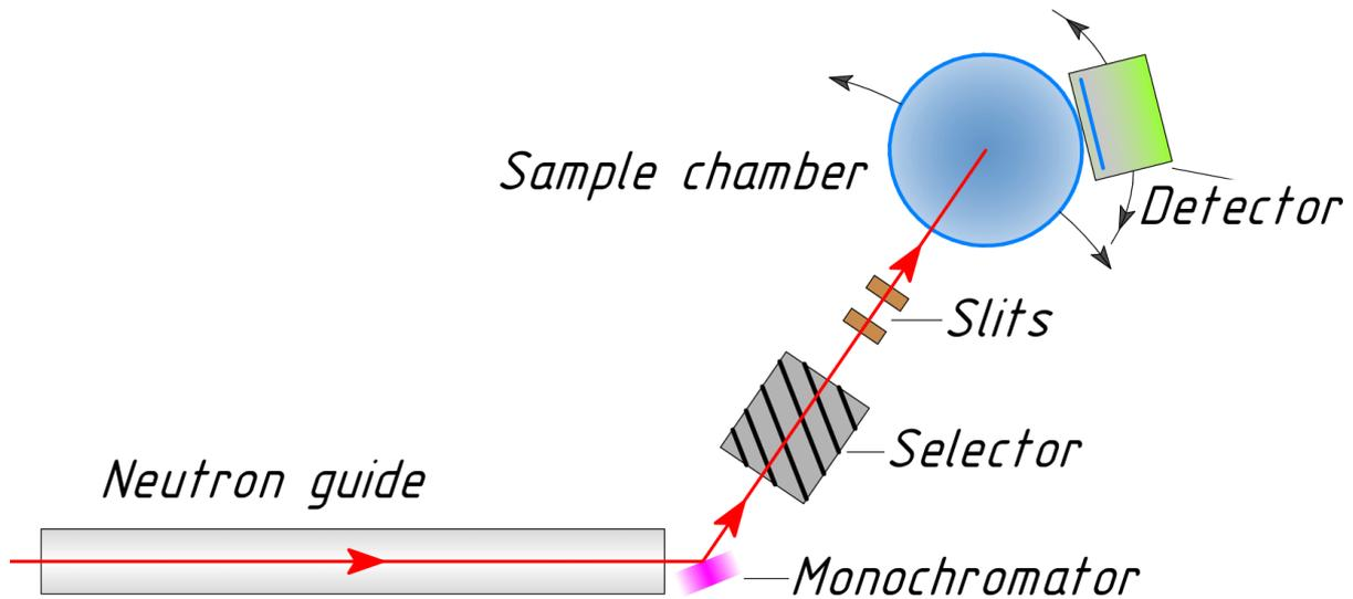
Fig. 2. BIODIFF instrument layout
