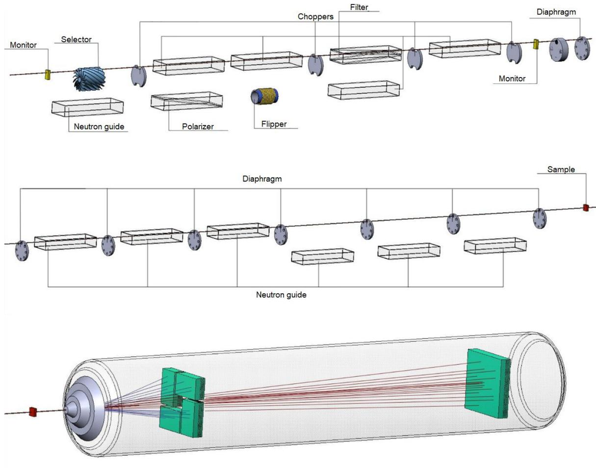
Fig. 3. MEMBRANA Instrument layout
