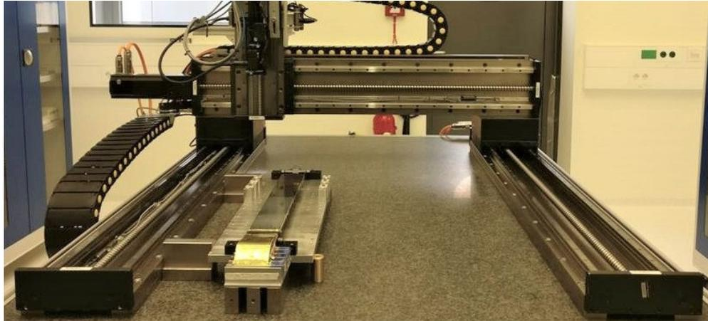
Figure 16 Station for ladder geometrical survey by optical means, with a ladder installed.
