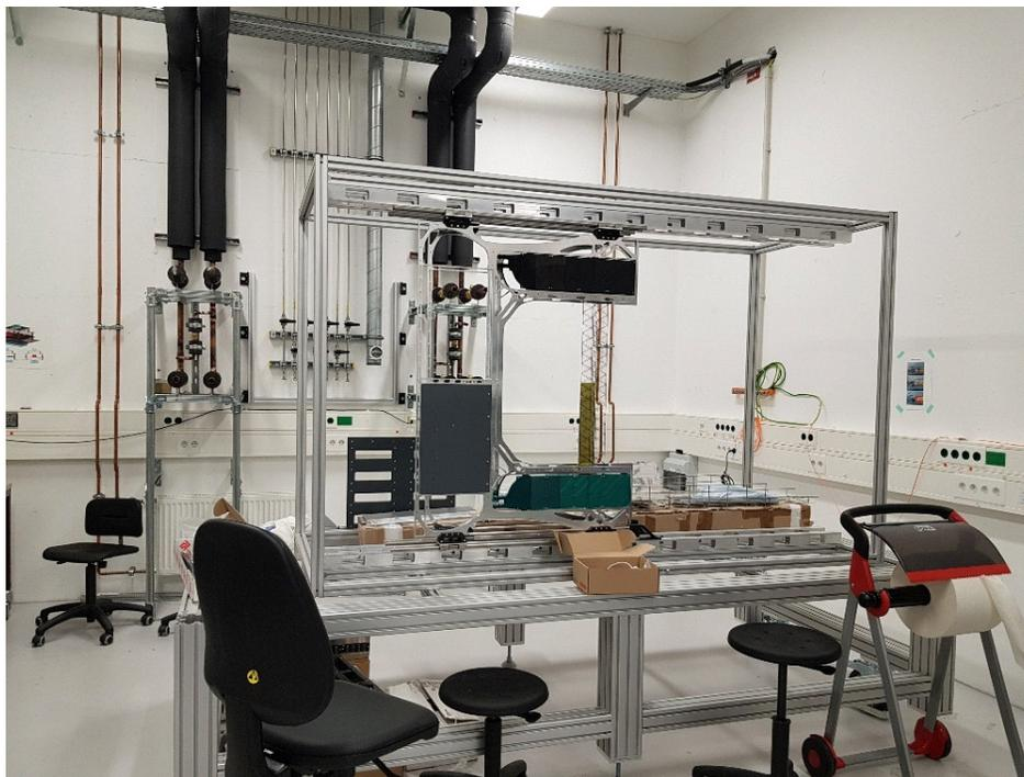
Figure 23 View into the emerging STS integration laboratory at GSI with a mechanical demonstrator of the STS mainframe on the assembly stand and some test ladder components mounted on C-frames.
