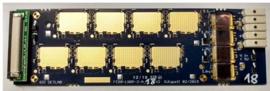
Figure 8 Front-end board equipped with passive components and connectors, ready for being used during module assembly.
