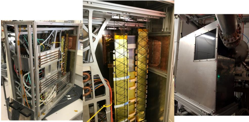
Figure 20 Views of the mSTS detector system after completed assembly. Detector ladders of the downstream stations (middle), C-frames with water-circulating cooling plates for the read-out boards visible installed in the detector mainframe (left), and closed detector box with the downstream particle window at the final installation point in the mCBM cave near the target and downstream beam pipe for the non-interacting beam.
