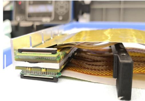
Figure 11 Assembled module (top). As the last step, the two front-end boards are attached to either sides of an L-shaped cooling fin (bottom). Finally, a shielding layer is attached on the outside faces of the module's microcable stacks.
