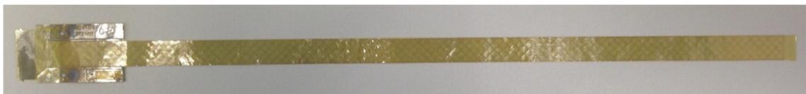
Figure 6 A microcable of 64 lines and a meshed Kapton spacer on top, with its „technological zone“ for testing, to be cut away before bonding to the sensor (left), and bond area to the ASIC (right).
