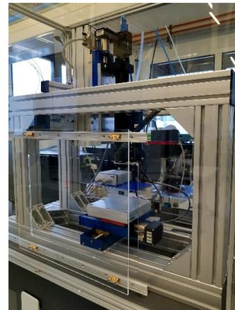
Figure 2 Optical inspection station from EKUT located in a clean room of the GSI Detector Laboratory.
