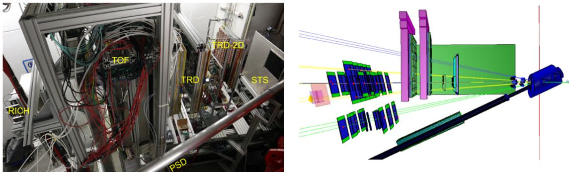
Figure 19 mCBM demonstrator experiment: Photo in the cave (left); detector geometry (right). The mSTS detector is installed downstream of the target and receives secondary particles produced at the target and sprayed out under CBM aperture angles between 2.5 and 25 degrees with respect to the non-interacting beam particle.
