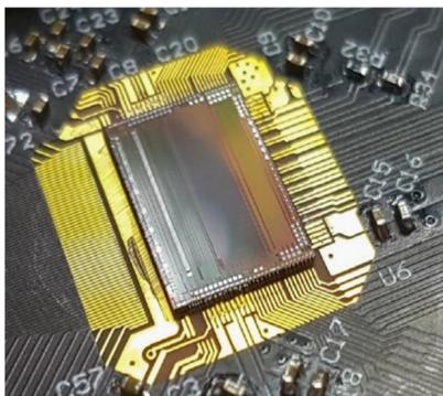
Figure 3 STS-XYTERv2.2 ASIC on a test board.
