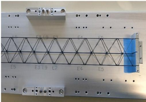
Figure 14 Carbon fiber ladder structure produced from fiber roving and fiber rods, installed on an assembly fixture.
