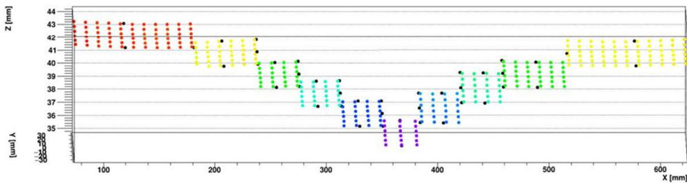
Figure 17 Survey results showing the height profile of the modules' silicon sensors mounted on the carbon fiber support.
