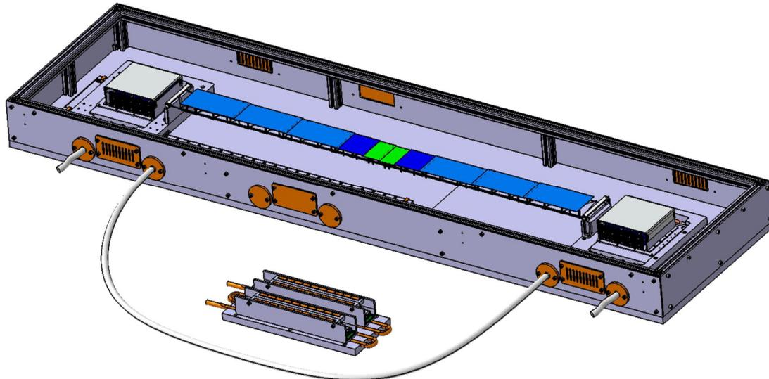
Figure 18 Depiction of a ladder test box, allowing to operate the modules on the ladder with its front-end electronics boards installed in the two boxes to its left and right ends, which are attached to cooling plates to remove dissipated power. The required power supplies and read-out electronics is operated outside of the box and is interfaced through connectors in the walls of the box.
