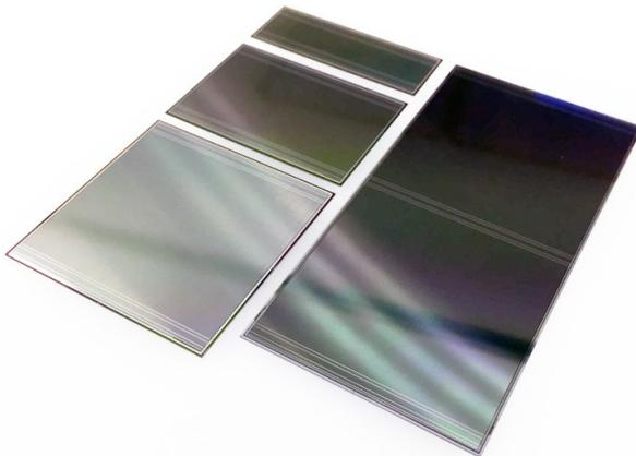
Figure 1 The four variants of the CBM-STs silicon microstrip sensors, accommodating on 6.2 cm width 1024 channels at 58  $\mu\text{m}$  pitch, in 2, 4, 6 and 12 cm strip lengths.
