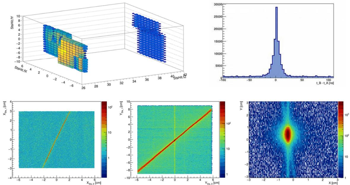
Figure 21 Results emerging from mSTS data reconstruction (*preliminary*): Space distribution of reconstructed hits (top left), time distribution with respect to Time-of-Flight detector hits (top right), X,Y correlation of STS hits in Stations 1 and 2 (bottom left), and extrapolation of the vertex in the target plane (bottom right).
