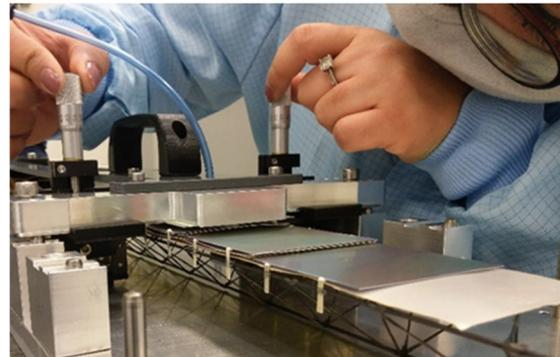
Figure 15 Specialized tooling allows installing one-by-one the modules onto the carbon fiber frame, thus yielding a detector ladder.
