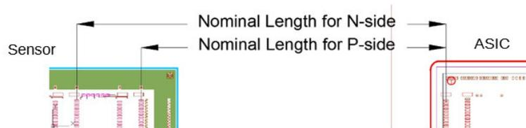
Figure 5 Principle of microcable line routing between contact pads on the silicon sensor and the ASIC, for p- and n-side connections and separated on two sub-cables connecting to two staggered contact rows with even- and odd numbered channel numbers. The cable lengths are between 160 and 495 mm.
