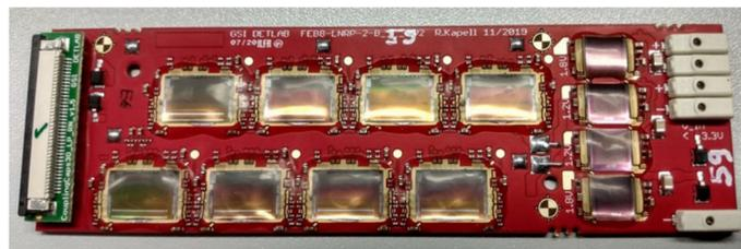
Figure 4 Eight STS-XYTER ASICs on a prototype Front-end electronics board FEB8-2 prepared for functionality tests. It comprises also four power regulating LDO ASICs custom-developed for CBM.
