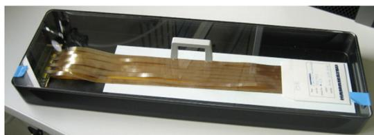
Figure 12 Completed module, prior to shield layer attachment, in a temporary storage box.
