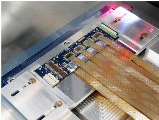
Figure 10 Chip cables aligned on a support structure for sub-sequent attachment to the silicon microstrip sensor, also via TAB bonding. This procedure is done in two steps of 8 chip cables each to complete one sensor side; then the assembly has to be turned over for attachment of the chip cables to the back side of the sensor (top). Finally, the ASICs are installed into two Front-end boards, one board per module side (bottom).
