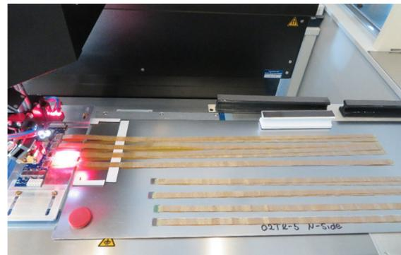
Figure 9 Initial Module assembly step: Attachment of STS-XYTER ASICs via TAB bonding to microcables, yielding “chip cables”.
